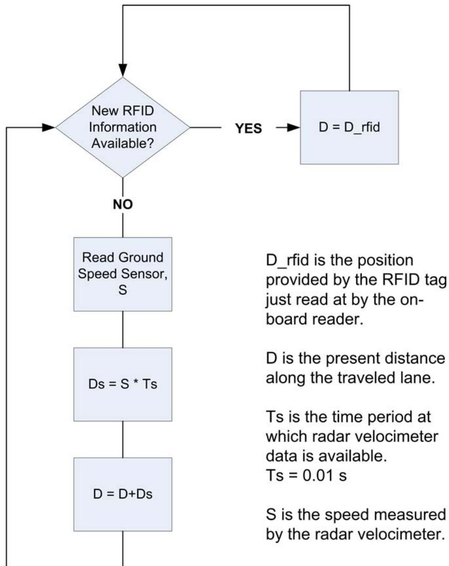
**Figure 4. Flow chart for determining position along the lane of travel using VPS and on-board radar velocimetry. GMH Engineering sensor provides speed measurements at a 100 Hz rate.**
