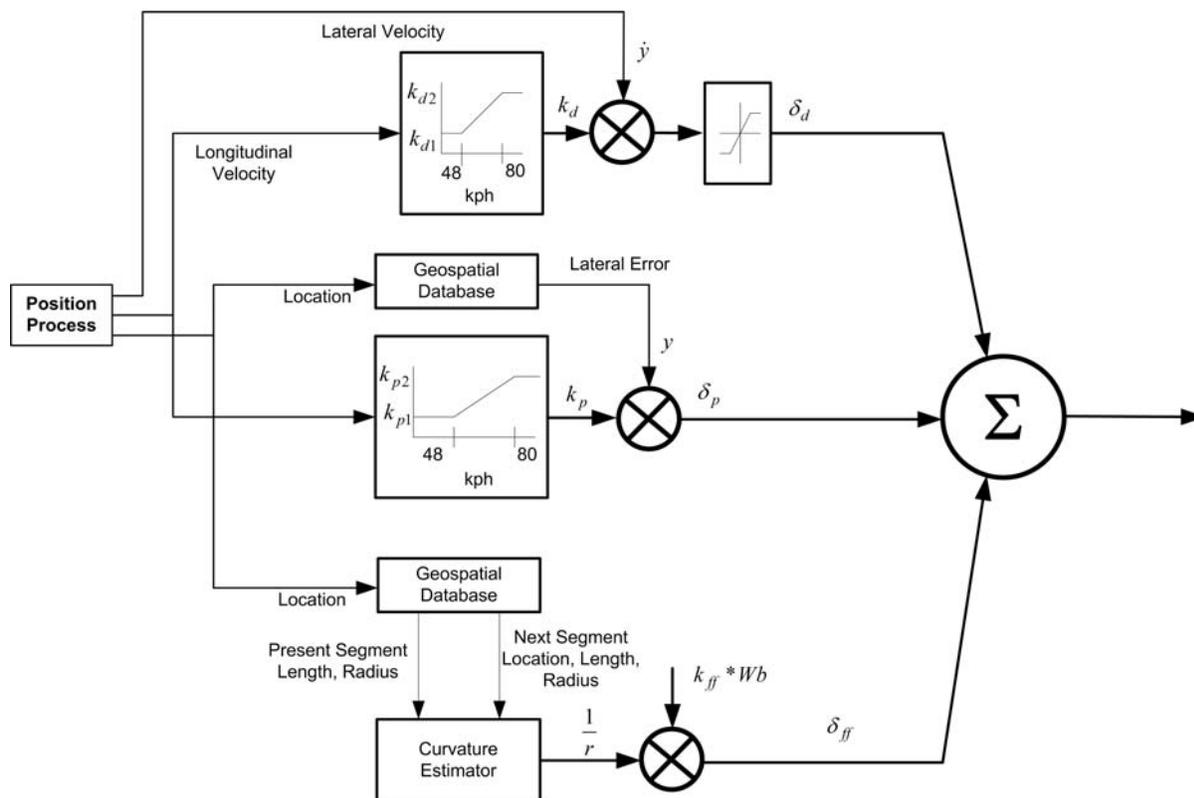
**Figure 10. Lateral control algorithm for providing lateral lane assistance. Key feedback includes lateral position, lateral velocity, and road curvature. These three elements can be extracted from the VPS-Laser Scanner system, allowing the same control algorithm to be used for either DGPS- or VPS-based guidance.**
