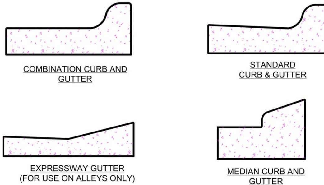
**Figure 6. A few example cross-sections of various curb geometries used in the US. For cross-correlation methods, sharp corners represent the preferred geometry. However, with a proper curb model, the cross-correlation techniques can prove robust.**
