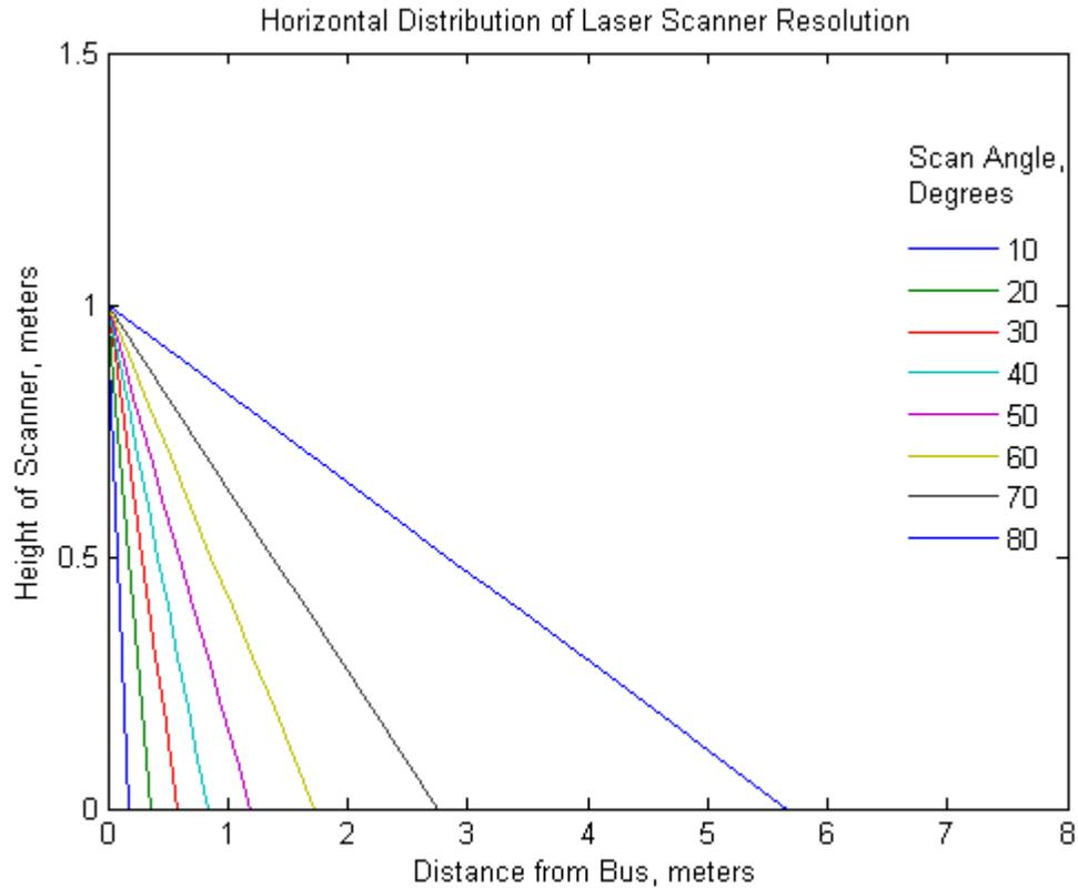
**Figure 9. Horizontal distribution of the vertically mounted laser scanner used to detect the presence and location of curbs used to determine bus lateral position within a lane. The greater the distance from the curb, the lower the resolution of the laser scanner in the direction of the horizon.**
