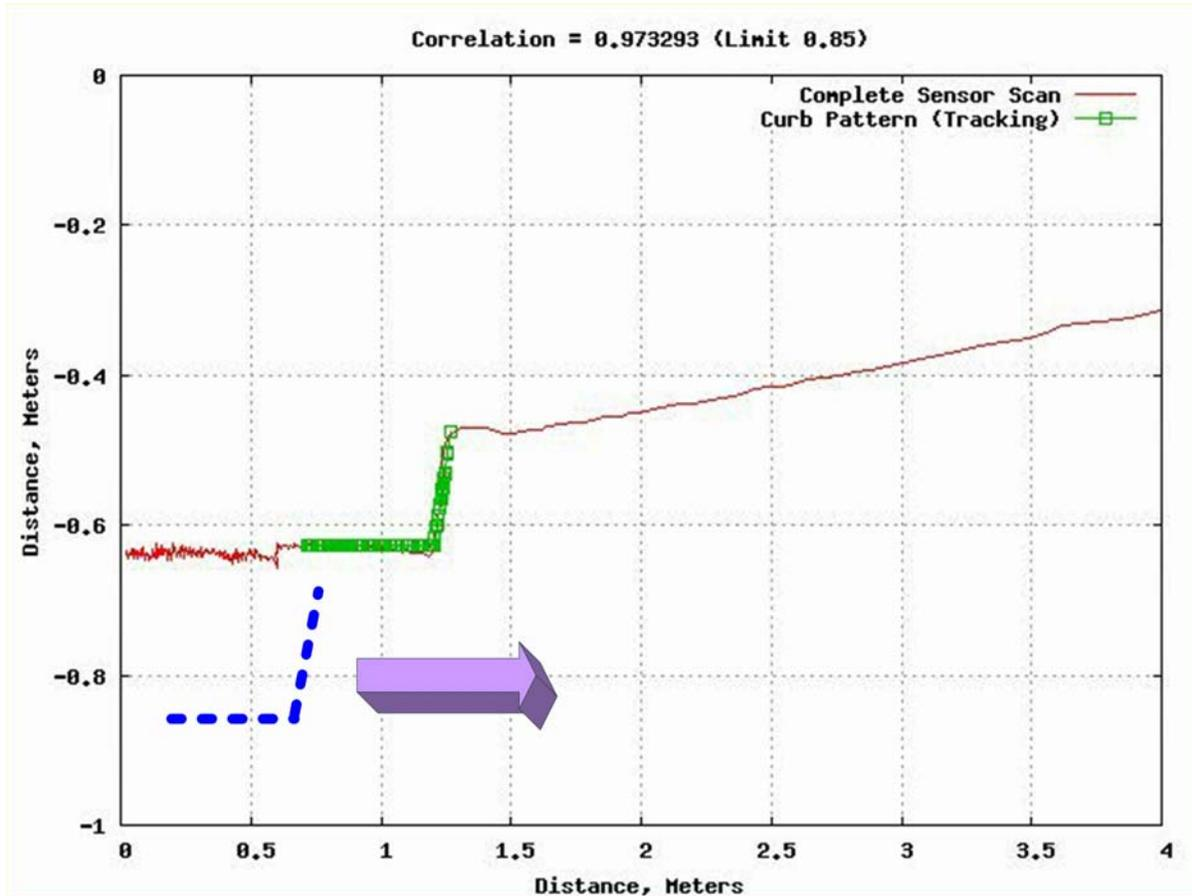
**Figure 8. Cross-correlation example for a square curb using a curb profile captured with laser scanner data. In this example, the peak normalized cross-correlation value is 0.973, and occurs at a distance of approximately 1.2 meters from the right edge of the bus.**
