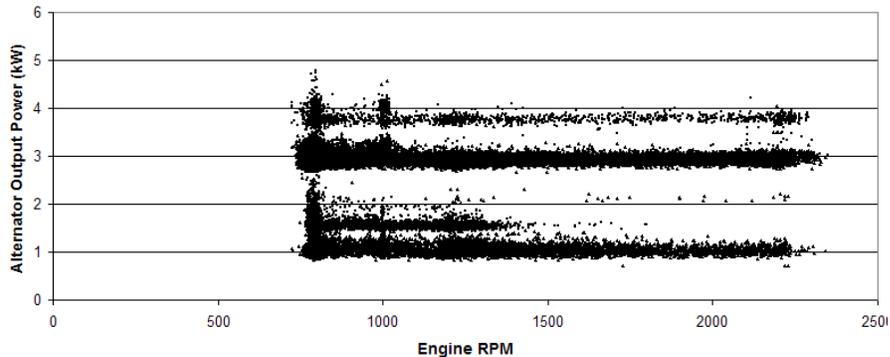
**Figure 23: Alternator Output Power vs. Engine RPM**
