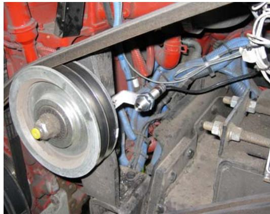
**Figure 4: Idler and Optical Sensor**
