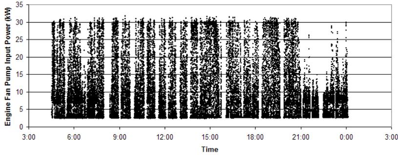
**Figure 12: Engine Fan Input Power Time Series**
