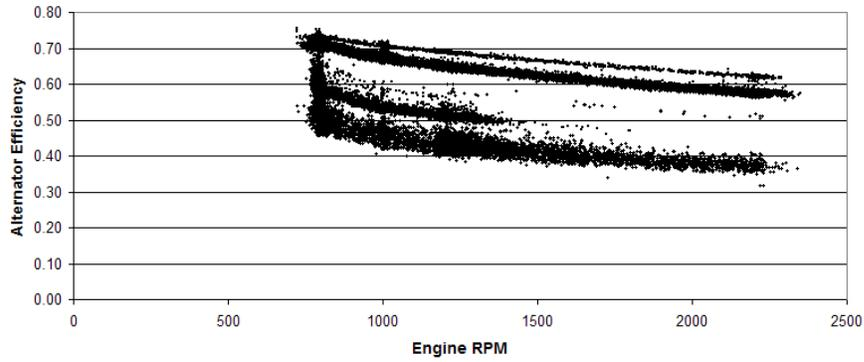
**Figure 24: Alternator Efficiency vs. Engine RPM**
