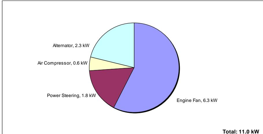
**Figure 28: Average Accessory Input Power (kW): Air Conditioning Off**
