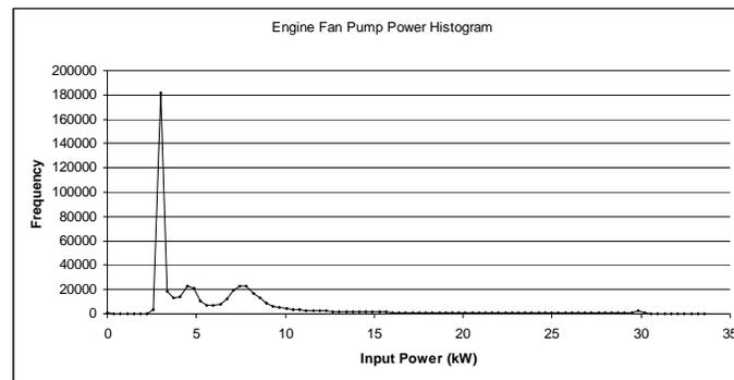
**Figure 15: Engine Fan Input Power Histogram**
