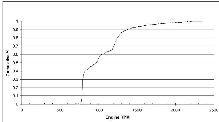
**Figure 11: Cumulative Engine RPM Histogram**
