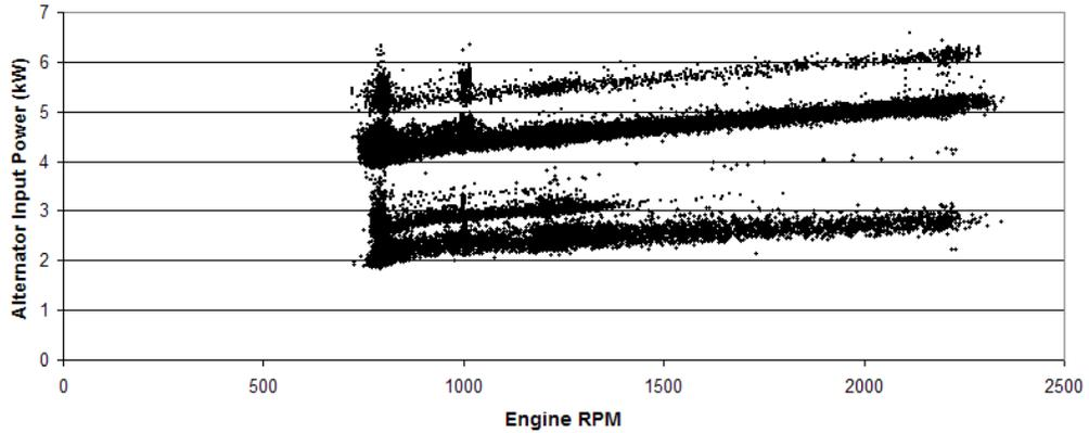
**Figure 22: Alternator Input Power vs. Engine RPM**
