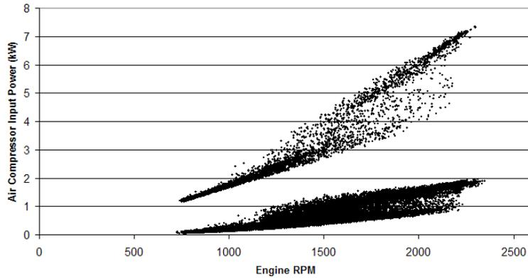
**Figure 20: Air Compressor Input Power vs. Engine RPM**
