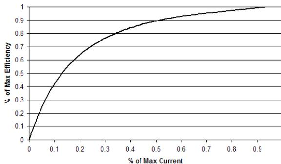
Figure 7: Alternator Efficiency Normalization
