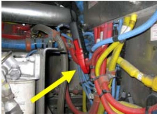
Figure 6: Alternator Current Sensor
