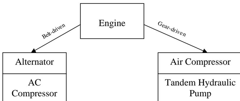
**Figure 3: Accessory Schematic**
