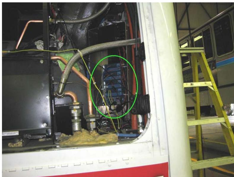
**Figure 2: Compact FieldPoint Data Acquisition System**
