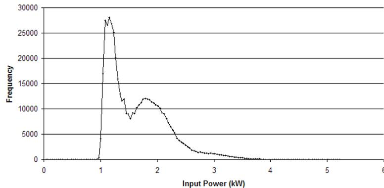
**Figure 17: Power Steering Pump Input Power Histogram**
