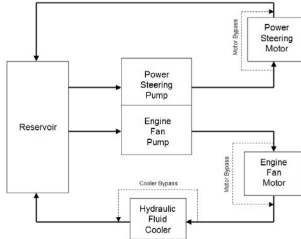
**Figure 5: Hydraulic System Diagram**
