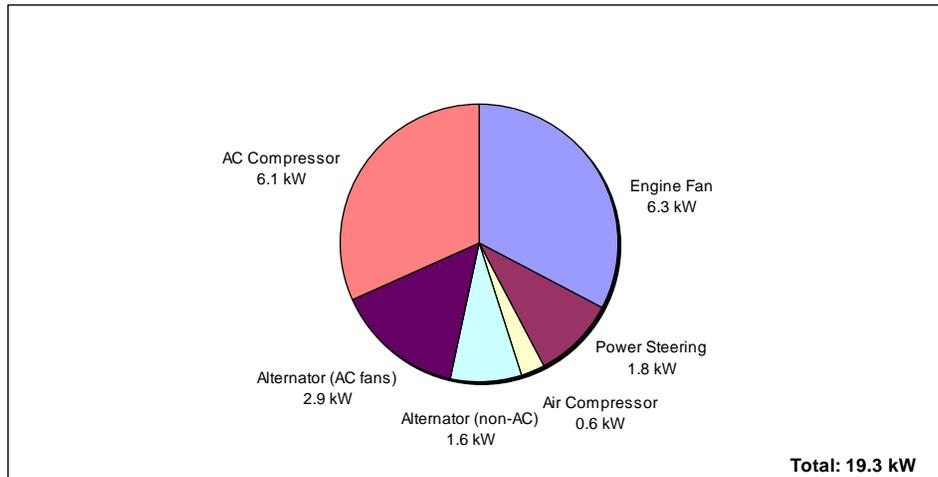
**Figure 29: Average Accessory Input Power (kW): Air Conditioning On**
