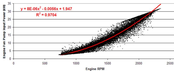
**Figure 13: Engine Fan Pump Input Power vs. Engine RPM**
