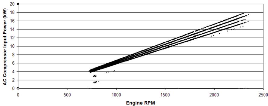
**Figure 18: AC Compressor Input Power vs. Engine RPM**
