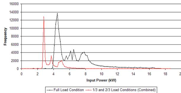
**Figure 19: AC Compressor Input Power Histogram**
