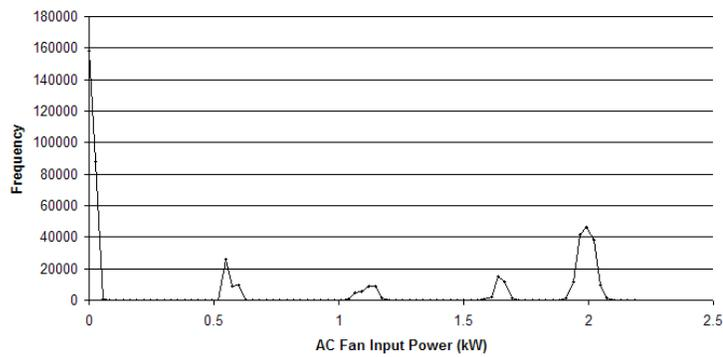
**Figure 25: AC Fan Input Power Histogram**
