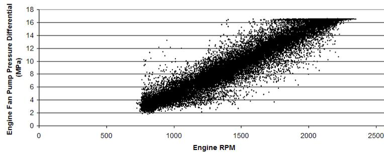
**Figure 14: Engine Fan Pump Pressure Differential vs. Engine RPM**
