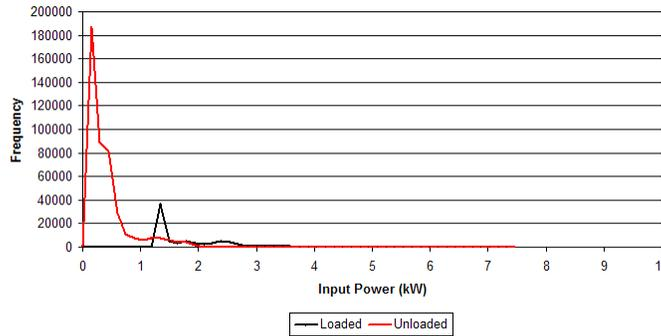
**Figure 21: Air Compressor Input Power Histogram**
