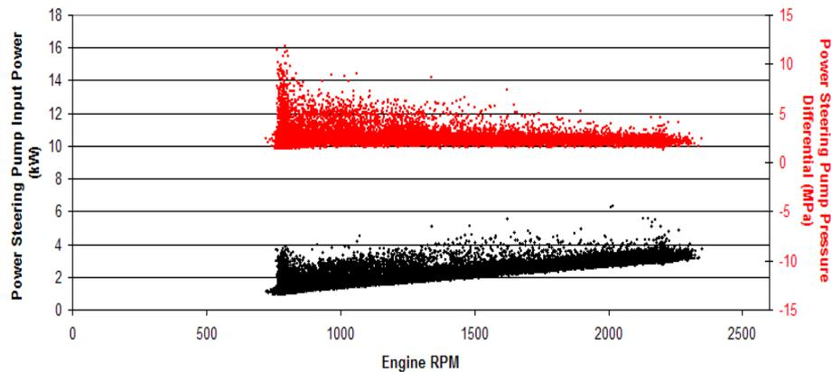
**Figure 16: Power Steering Input Power, Pressure Differential vs. Engine RPM**
