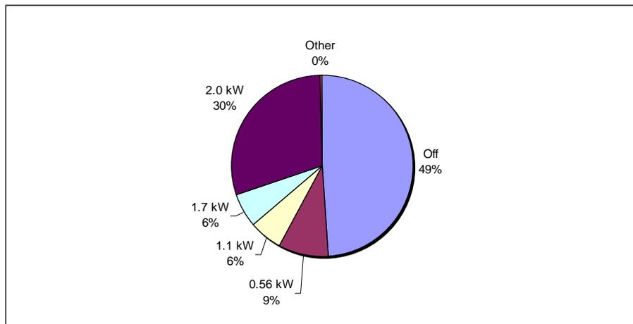
**Figure 26: Relative Frequency of AC Fan Power Settings**
