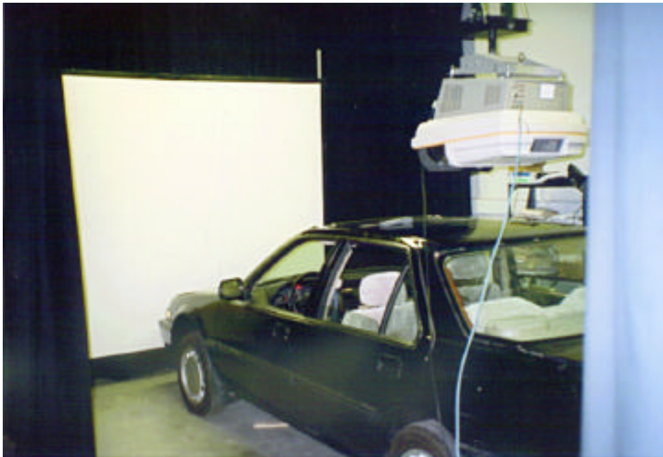
Figure 2.1. Human Factors Research Laboratory's Front-Projection Driving Simulator
