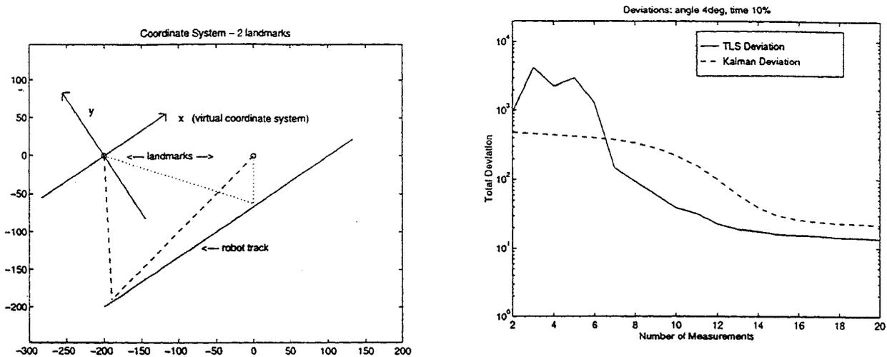
Figure 4: *Obtaining location from vision data: the geometric setup (left), typical performance results (right).*
