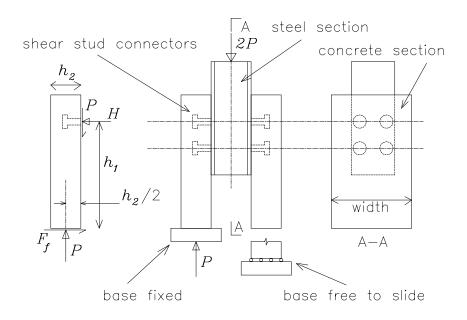
Figure A.2: Conventional Push-Out Specimen [after (Oehlers and Bradford, 1995)]
