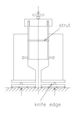
Figure A.3: Modified Push-Out Specimen [after (Oehlers and Bradford, 1995)]
