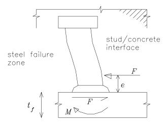
Figure A.1: Stud Shear Connector in a Composite Member [after (Oehlers and Bradford, 1995)]
