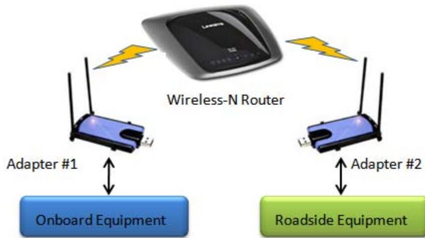
Figure 2.11 Wireless Communications Using the WUSB-N Wireless Adapter and Router
