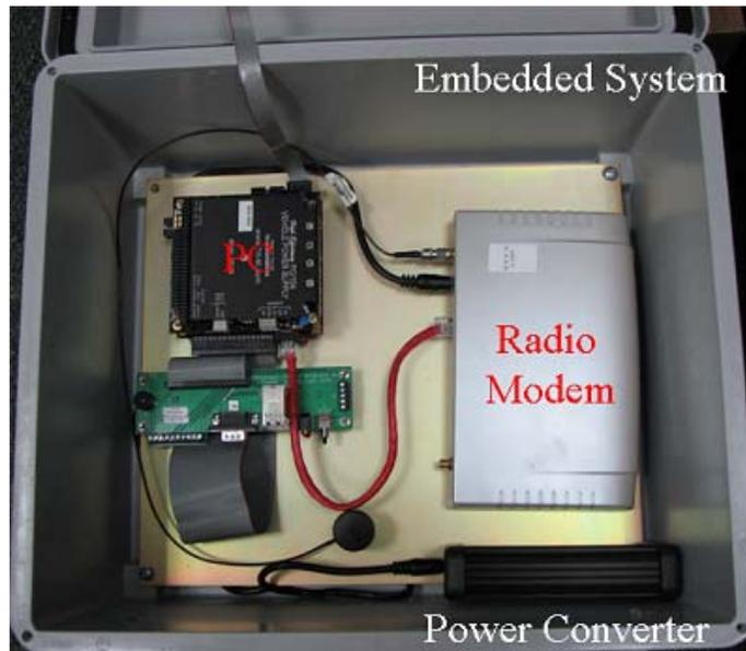
Figure 2.13 The Embedded Signal Priority System Packaged in a NEMA Enclosure
