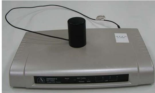
Figure 2.4 Denso DSRC Wireless Modem
