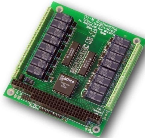
Figure 2.2 R104-88 Optoisolated Input and Relay Output Board
