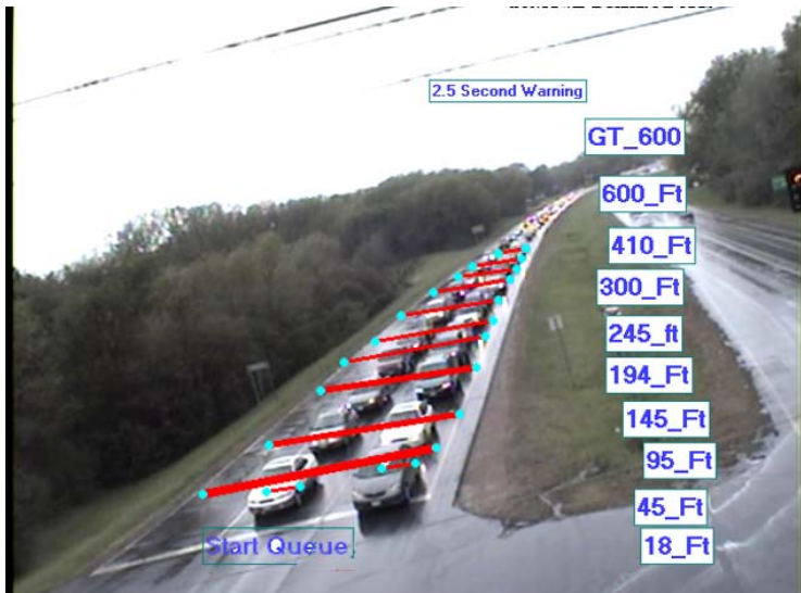
Figure 1. Presence detector ‘ladder’ configuration of algorithm used to detect the onset of queues, queue length, and queue warning alarm trigger.
