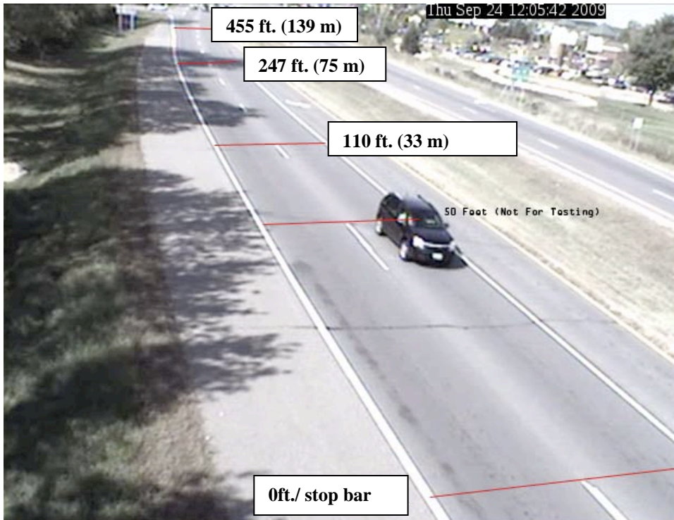
Figure 8. Front of queue and length measures at HWY 55 & Rhode Island Ave. intersection used for ground truth observations.
