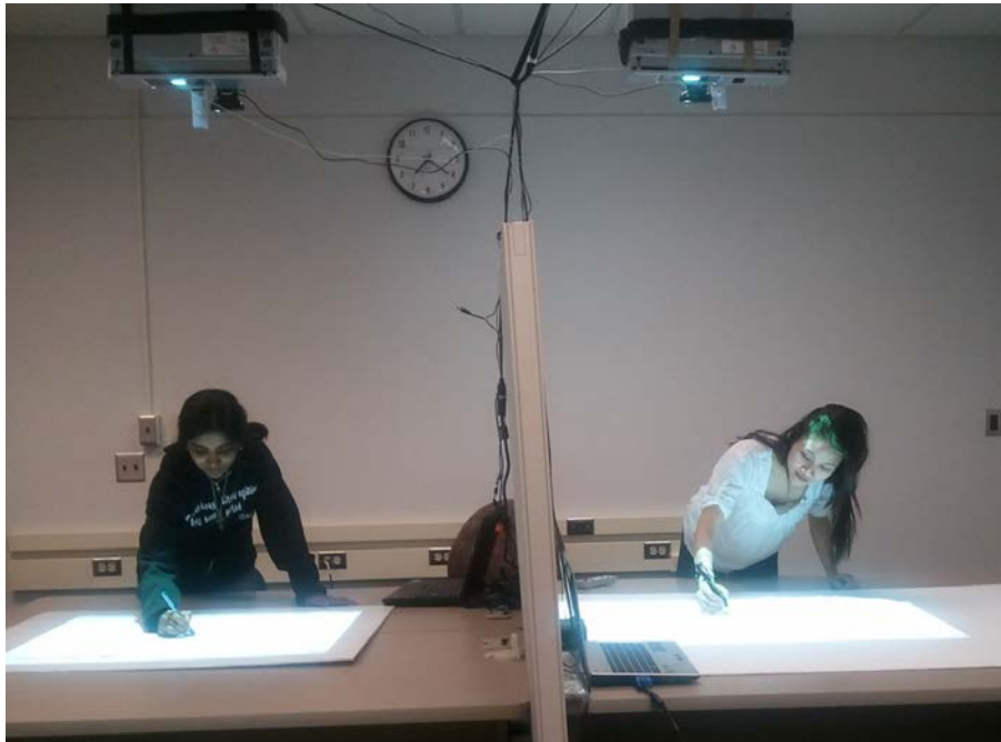
Figure 1: Two of the software developers demonstrate virtual collaboration on a shared electronic map. They are separated by a soft wall; they can hear but not see each other (except through the interface). Each side has a projector, infrared sensor, and camera directed at an ordinary conference table. Participants control the application using the infrared pens in their hands.
