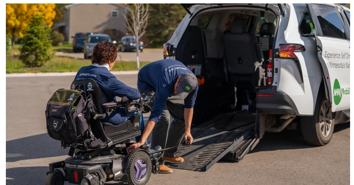
Of the five goMARTI project vehicles, three are equipped to accommodate a passenger who uses a wheelchair.
