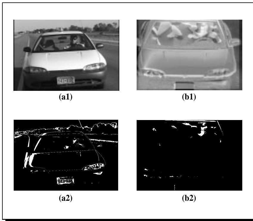
Figure 1.19: Comparative results between the visible spectrum approach and the near-infrared fusion approach.
