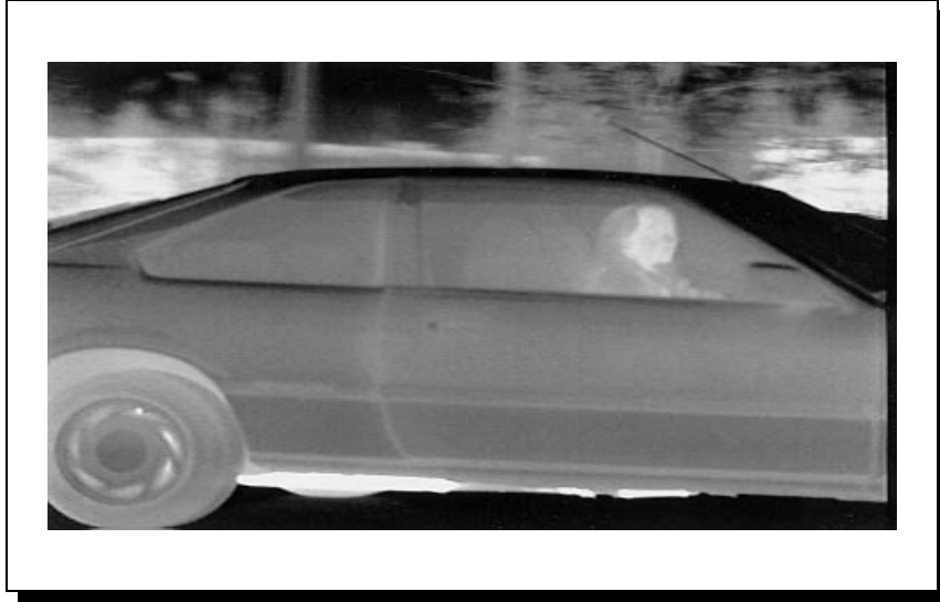
Figure 1.5: Side snapshot of a low speed car with a mid-infrared camera.
