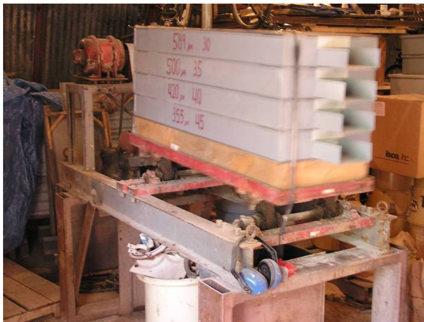
Figure A.2: Use of a rectangular sieve shaker table and customized screens increased productivity significantly over commonly used Ro-Tap shakers.
