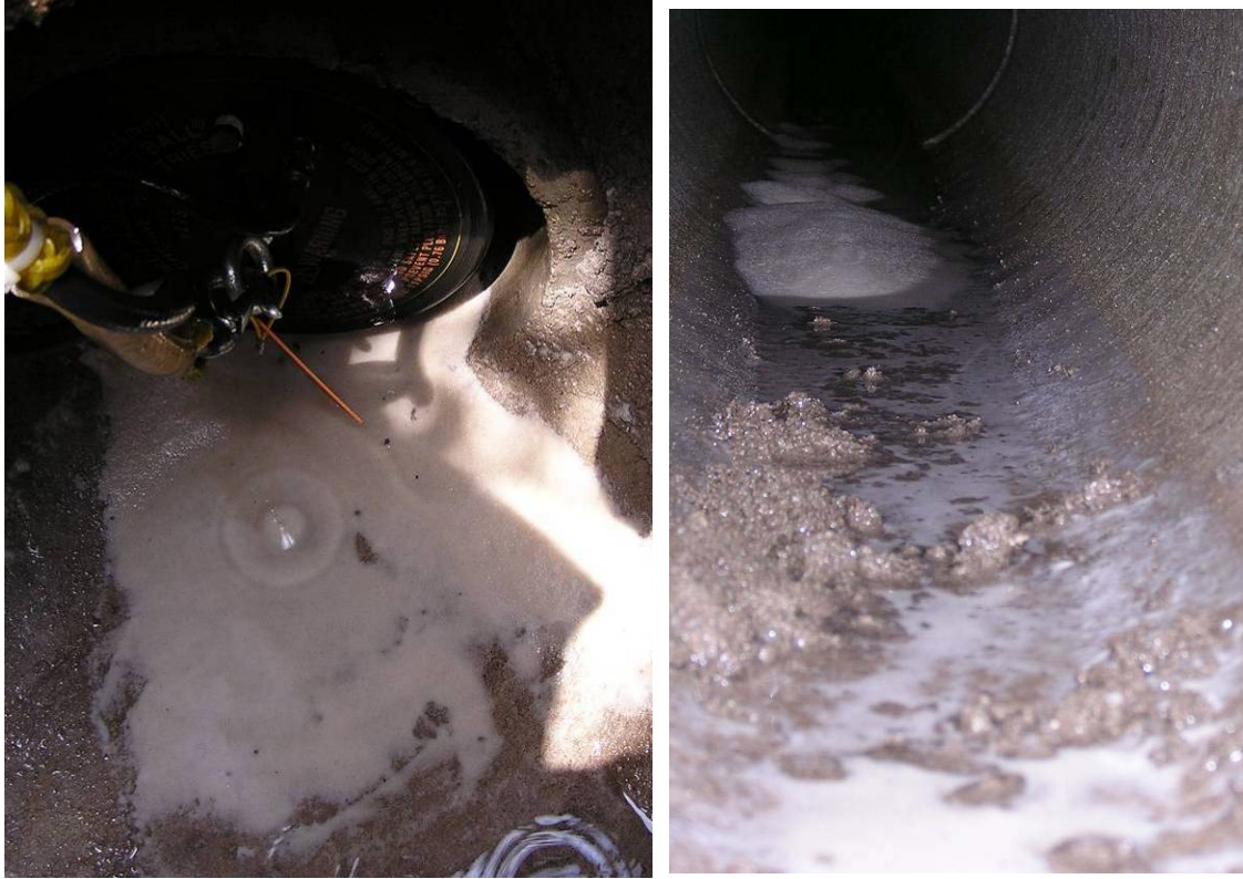
Figure C.14: Results of trial sediment feeding location 100 feet upstream of the Vortechs System. Sand settling in manhole in which it was fed (left) and along the 100-foot reach of the pipe leading to the Vortechs System (right).
