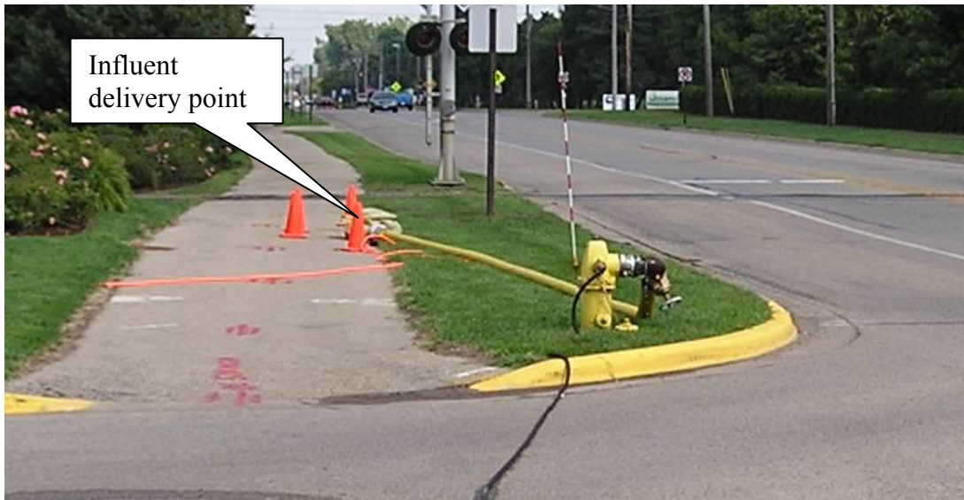
Figure C.19: Influent piping configuration, making use of the same hydrant fittings as at previous testing sites and a reach of fire hose to cover the ~10 m (35 ft) from hydrant to influent delivery point.
