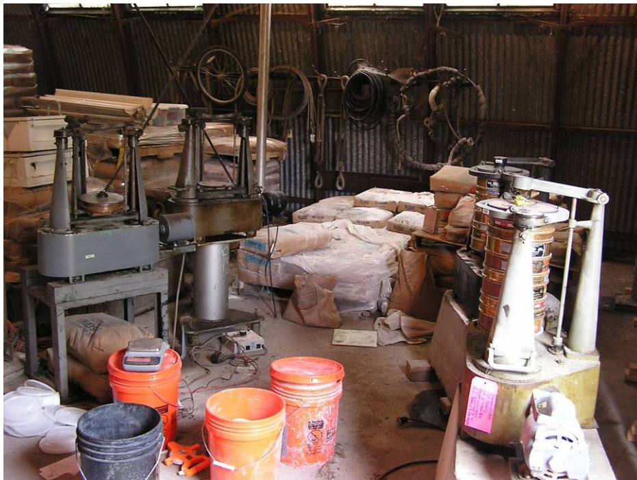
Figure A.1: Four Ro-Tap sieve shakers were relocated to the Quonset hut adjacent to SAFL to maximize operator productivity
