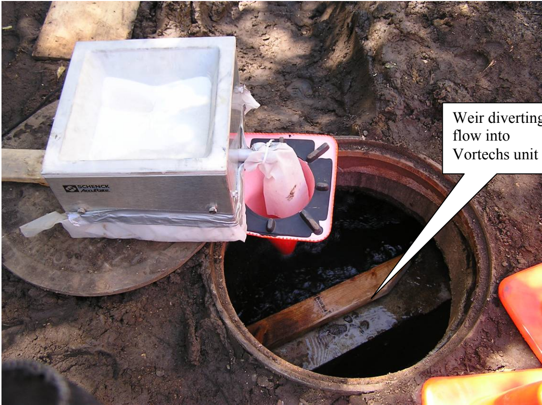
Figure C.15: Sediment feeding location at STMH3B.
