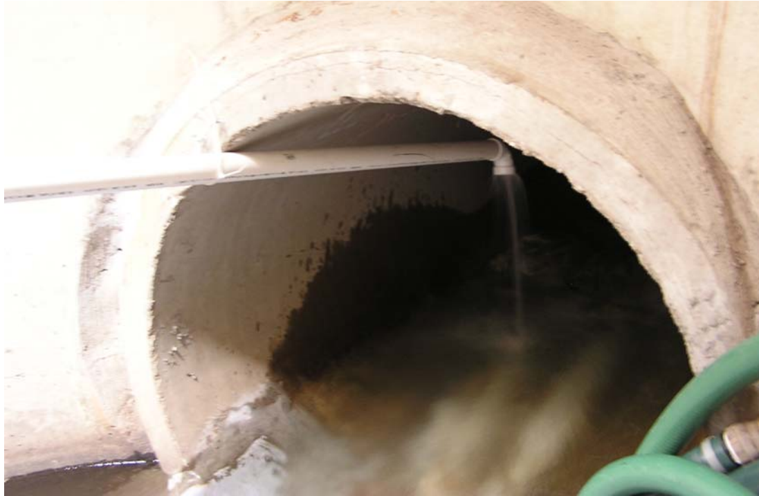
Figure C.21: Downstream end of the sediment delivery piping system approximately 1.8 m (6 ft) upstream of the Stormceptor. A 90° elbow at the downstream end helped direct the flow to the centerline of the storm drain pipe for conveyance into the device.
