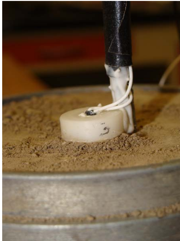
Figure 5. Button heat pulse sensor reading temperature rise on soil packed in AASHTO T99 mold.
