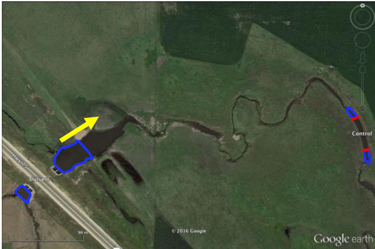
Figure 2.3 Satellite image (Google Earth) of Poplar Creek with culvert 59X09 and corresponding control area. Imagery taken 05/2015. Image shows pool upstream and downstream of culvert and the two tributaries upstream of the culvert. Blue delineates fish sampling areas, and red lines show the control stream reach. Flow direction is shown by the yellow arrow.
