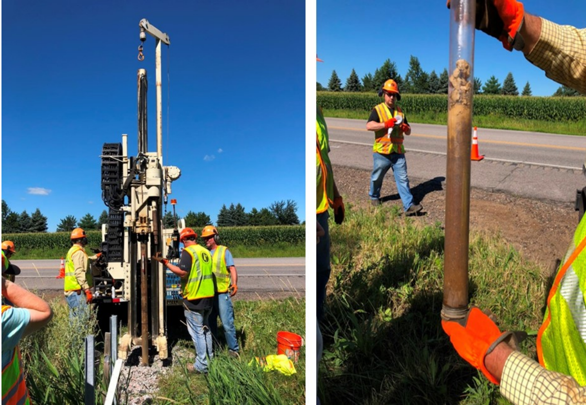
Figure 6.5. Filter media core collection using a Geoprobe® at the iron-enhanced ditch check in July 2018.
