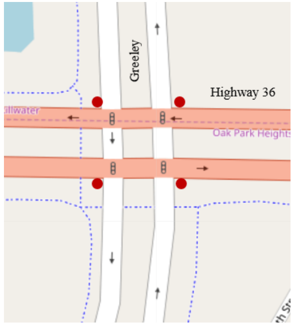
Figure 2.12 Location of Bluetooth Beacons Installed at Highway 36 and Greeley Intersection. (Background Image from OpenStreetMap, 2020)
