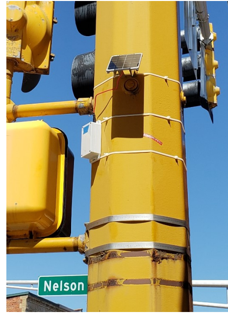
Figure 2.10 Images of Bluetooth Devices Attached to Signal Poles at Nelson St.
