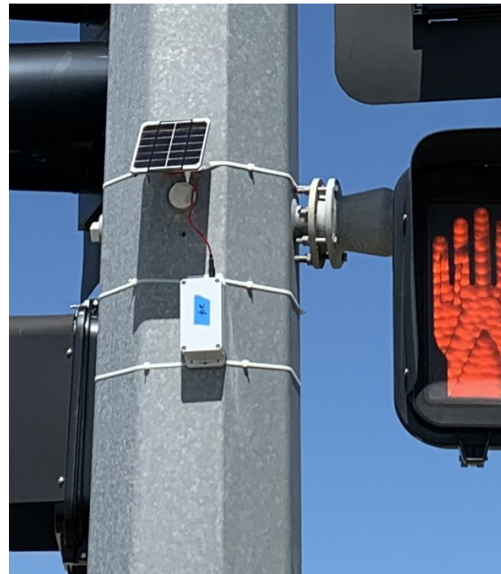
Figure 2.11 Images of Bluetooth Devices Attached to Signal Poles at Greeley & Hwy 36.
