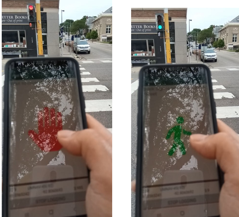
Figure 4.1 Snapshots of a video recording pedestrian walk phase transitions.
